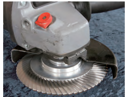
Rear view of an angle grinder with a weld root opener
